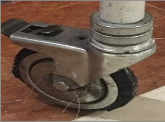
Weighing chair wheels found broken, it is imbalance and high risk for fall
